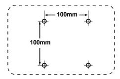
**Step 5.** Attach the LCD display to the wall, following the instructions in the wall-mounting kit.
